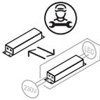
EN The LED driver contained in this fixture must only be replaced by the manufacturer, its support service or similarly qualified personnel.
